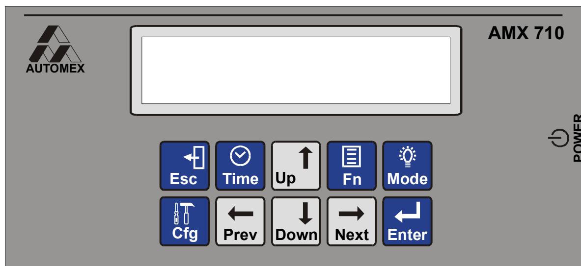
FIGURE 2. AMX 710 – the operator panel view.
